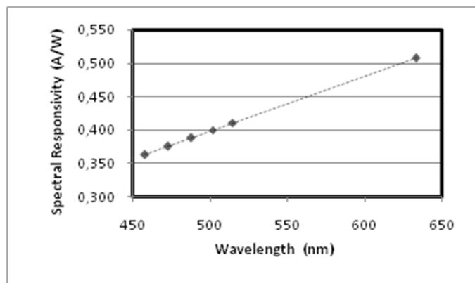
Fig. 1. Spectral responsivity of a trap silicon detector at some wavelengths of Ar<sup>+</sup> and HeNe lasers.
