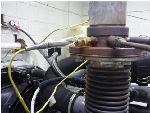
**Fig. 9. Thermocouple (exhaust gas' temperature)**
