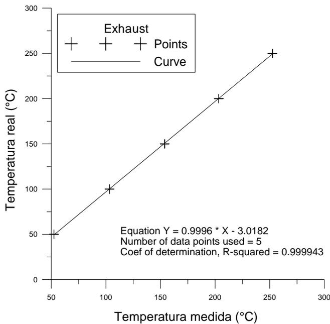
Fig. 18. Calibration chart for the thermocouple measuring the temperature of exhaust gases
