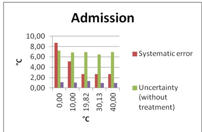
Fig. 13. Graph of errors in the measured points for thermocouple Admission
