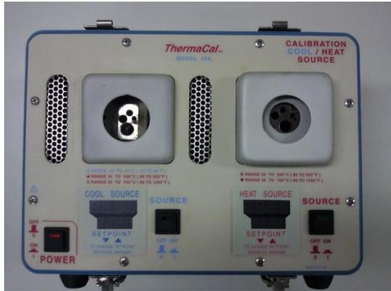
Fig. 10. Portable Calibrator of temperature sensors
