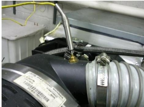
**Fig. 8. Thermocouple (air admission temperature)**
