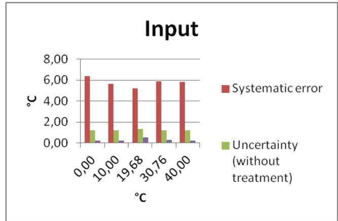
Fig. 12. Graph of errors in the measured points for thermocouple Input
