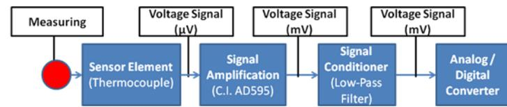
Fig. 2. Block Diagram of temperature measurement system
