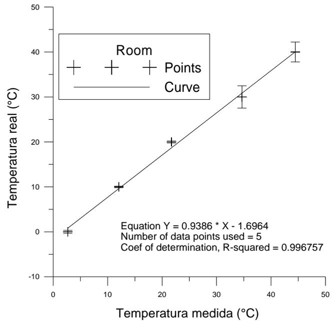
Fig. 15. Calibration chart for the thermocouple measuring the room temperature
