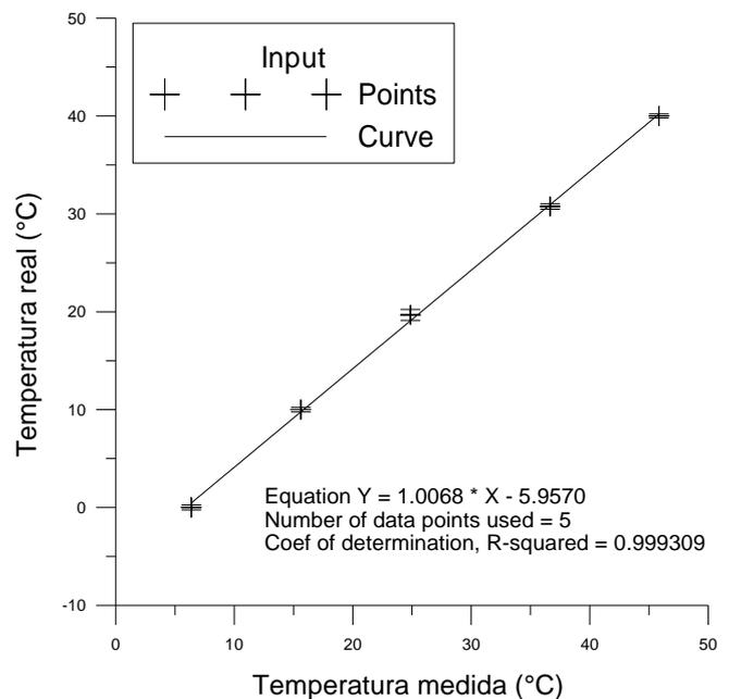
Fig. 16. Calibration chart for the thermocouple measuring the Input air temperature
