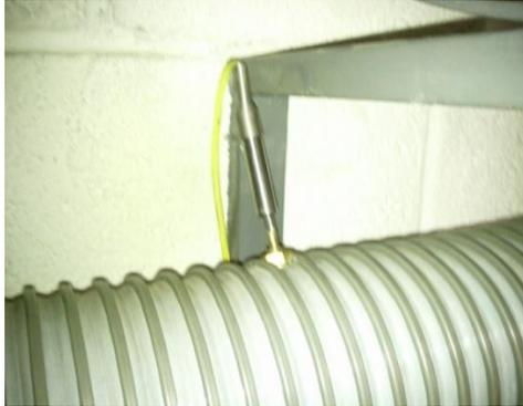
**Fig. 7. Thermocouple (air inlet temperature)**
