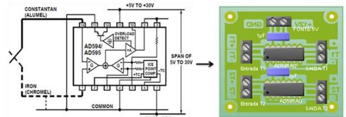
Fig. 3. Signal Amplifier Circuit
