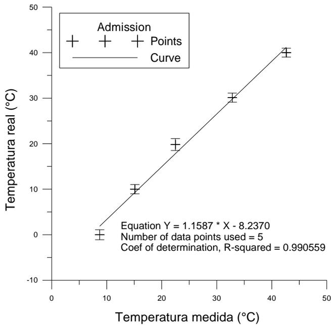
Fig. 17. Calibration chart for the thermocouple measuring the admission air temperature
