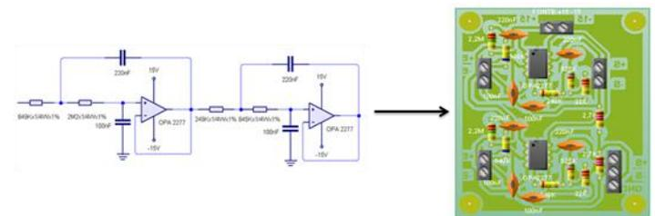
Fig. 4. Low-pass filter circuit
