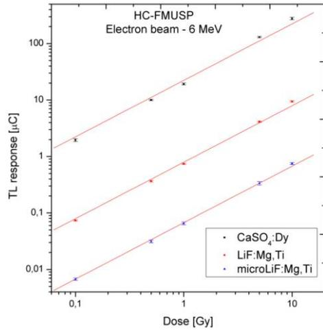
Fig. 5: Dose-response curves to 6 MeV electrons using solid water phantom.
