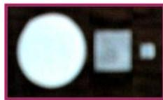
Fig.1. Thermoluminescent dosimeters of CaSO<sub>4</sub>:Dy, LiF:Mg,Ti and microLiF:Mg,Ti respectively.
