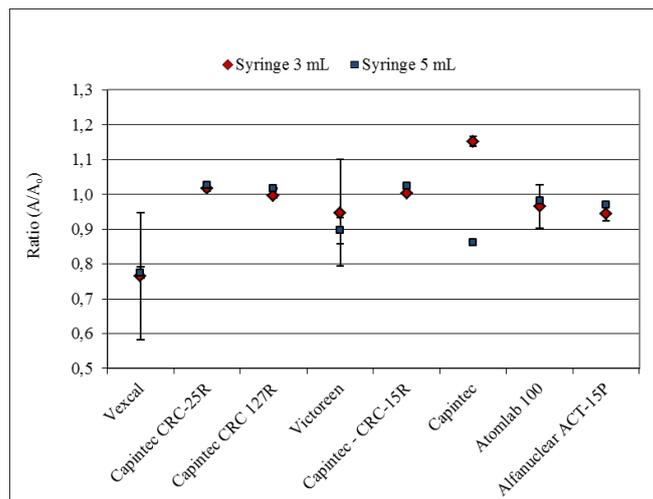
**Fig. 5 Comparison of activity measurements of  $^{99}\text{Tc}^m$  contained in plastic syringes**
