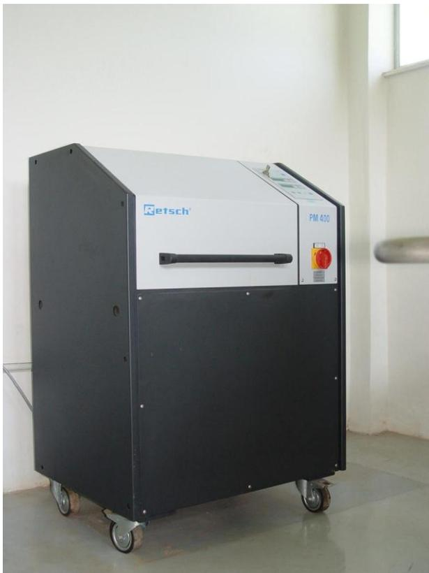
Fig. 1. Planetary Mill
