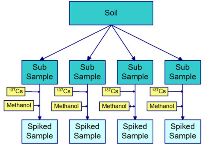
Fig. 5 Flowchart of soil individual method preparation
